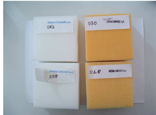
Fig. 3 Foam samples for the compression test.
